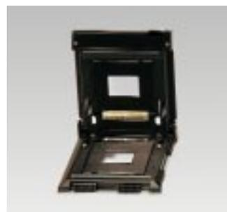
The professional film carrier is made of diecast aluminium, and features adjustable masking strips, register pins and automatic centering. With the aid of interchangeable metal masks and glass plates, the film carrier can be used for formats up to 6 x 7 cm (2 1/4 x 2 1/4 in) and APS.
